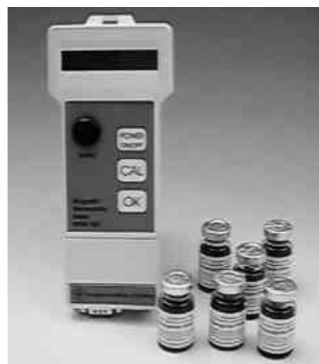
Fig. 1: The magnetic permeability meter used for the detection of human albumin.
