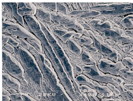
Fig. 4. SEM micrograph of alloy # B after the potentiodynamic polarization measurement.
