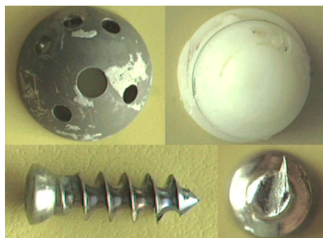
Fig. 1: Macroscopy view of the primary implant components who was analyzed: acetabular cup, polyethylene liner, screws.
