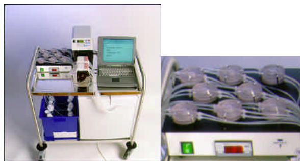
Fig. 2: Cart with warming plate, roller pump, laptop PC, refrigerator and waste bottles (left), close up of warming plate with 8 chambers (right).
