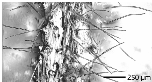
Fig. 2: Extended Focal Microscopy Imaging picture of a PHEMA leaf vein.
