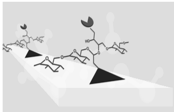
Fig. 1: Schematic representation of OptoDex ® based functional platform. After photo-immobilization photolinker polymer provides secondary functional groups (amino-, carboxyl-, maleimido-, activated thiol- or biotin functions, lactose or fluorophores) that modulate the physical properties of the surface, and/or enable binding (covalent or affinity) of probe molecules.
