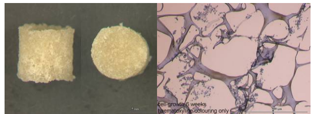
Fig.1: a) a porous, cylindrical scaffold, made with spider silk. B) Chondrocytes growing in the pores..
