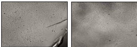
Fig. 1: Micrographs showing BAC (passage 2) after 7 days of culturing on (a) poly(NIPAM)-g-GMMA-co-EGDMA and (b)TCPS
