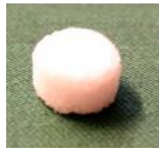
Figure 2. Sintered porous scaffold.
