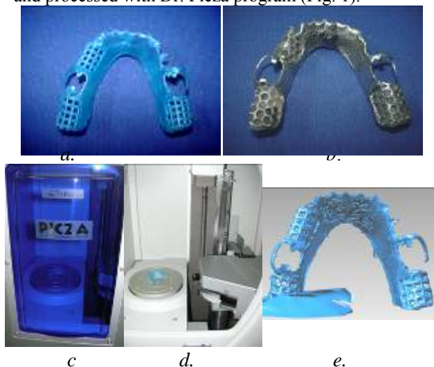
Fig.1 3D scanned wax pattern: a. “LiWa” wax pattern; b. metallic framework; c,d. scanner, e. 3D scanned wax pattern.
