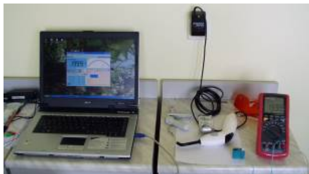
Fig.1. The measurement stand used in this study to measure the pulp chamber temperature.
