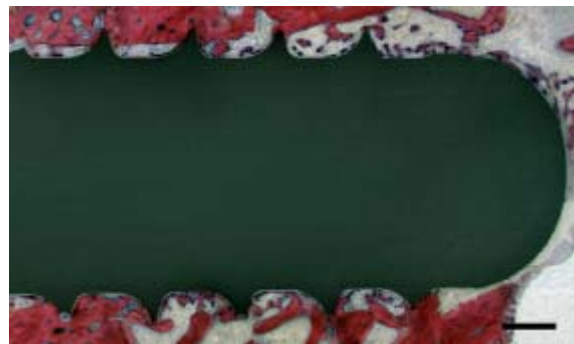
Fig. 2 Ceramic implant with surrounding bone. Note the newly formed bone within the threads. Giemsa/Eosin, scale bar = 600µm.
