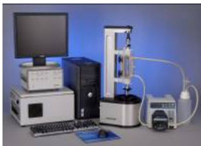
Figure 1. Biodynamic® system setup for hydrogel DMA tests
