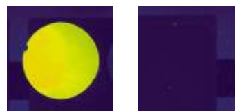
Fig. 1: Reactive amino groups on APTES treated (left) chip and negative control (right).
