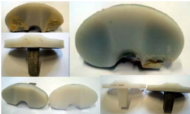
Fig.1: Example of some retrieved polyethylene components from knee prosthesis
