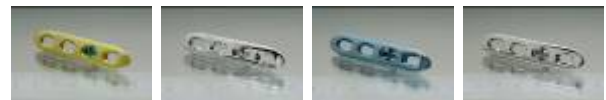
Fig.1. Constructs used included Std cpTi LCP/TAN screws; EP cpTi LCP/ TAN screws; PP cpTi LCP/ TAN screws; Ss LCP/ screws.
