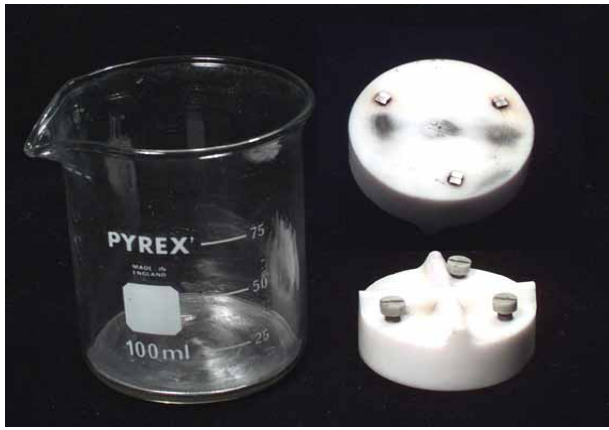
Figure 1. Particle generating apparatus. A disc of the appropriate metal is attached to the base of the beaker, by means of adhesive. The Teflon magnetic stirrer follower was modified to hold three pins of the metal, whose height above the surface could be adjusted by turning the plastic screws.
