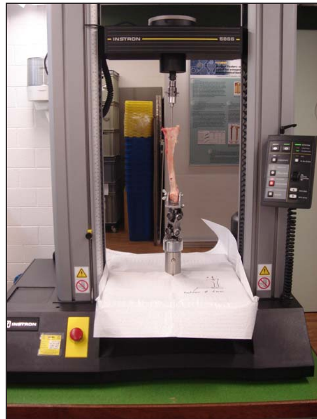
Figure 1. Testing Device, with adapter screwed into the endcap holder of the nail within the tibia before pull out with was performed with a constant force
